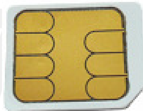
Sample of an 8 contact Mini UICC SIM card
